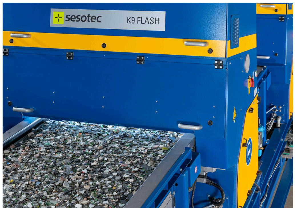
According to Glassco the facility is the „first of its kind“ and features high-speed cameras and state-of-the-art LED light technology for the detection of black glass.
