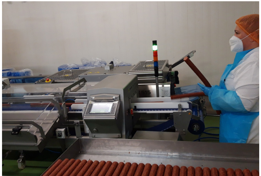
In order to detect debris from aluminum clips in unpackaged salami sticks, H. Loidl Sausage Producers and Distributors GmbH & Co uses INTUITY metal detectors with THiNK software from Sesotec.
