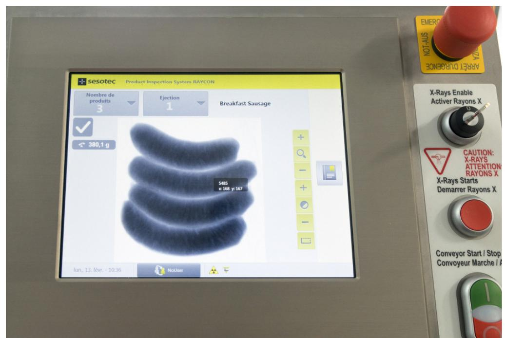
Along with performing its primary task of detecting foreign particles in the product flow, the RAYCON can also provide visual detection of misshaped products, as well as check for incorrect product weight.
