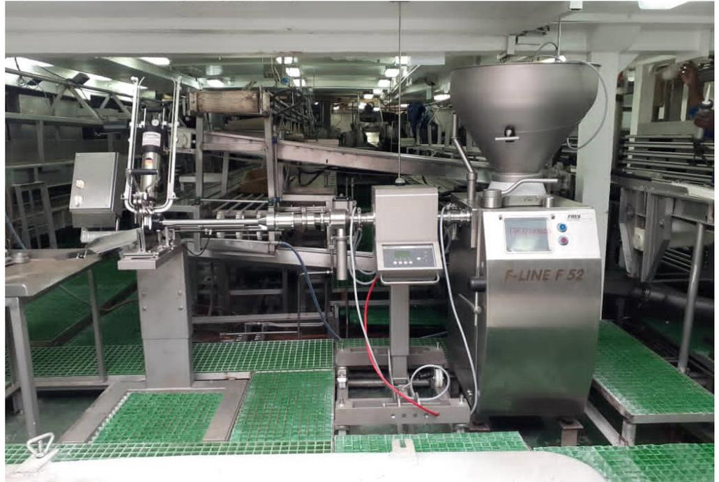
*Baader Namibia and Sesotec installed a metal separator directly into the production equipment on a fishing boat. Customer complaints about metal clips in fish sausages have ceased since implementing the LIQUISCAN VF+.*
