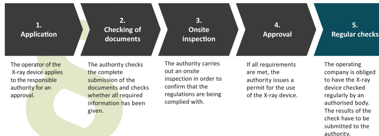
Practical example: the approval process according to the X-ray regulations (RöV) in Germany
