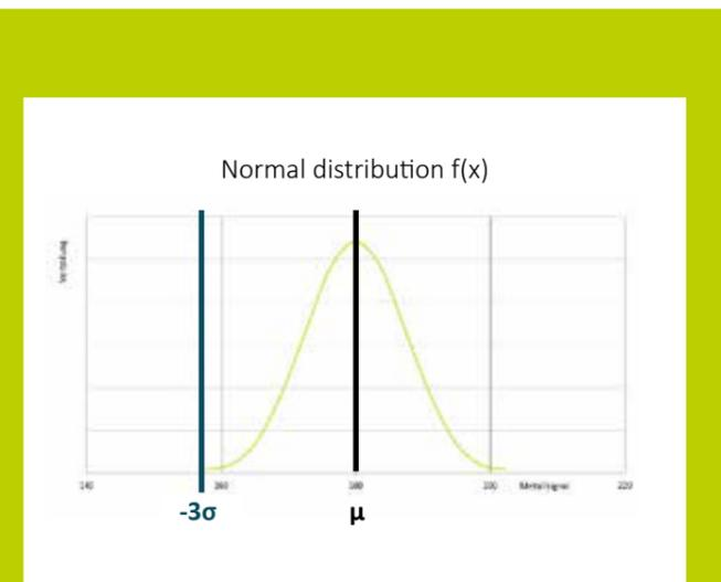
With a normal distribution, 99.73 % of all values lie in the range +/- 3 sigma ( $\sigma$ ) around the mean value  $\mu$ .  $-3\sigma$  is the lowest limit value for daily routine testing on site.
