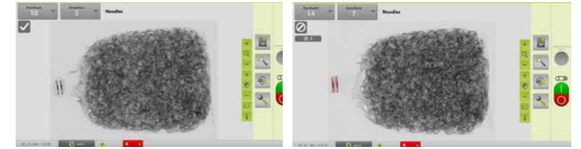
Ignoring metal clips to increase detection sensitivity
