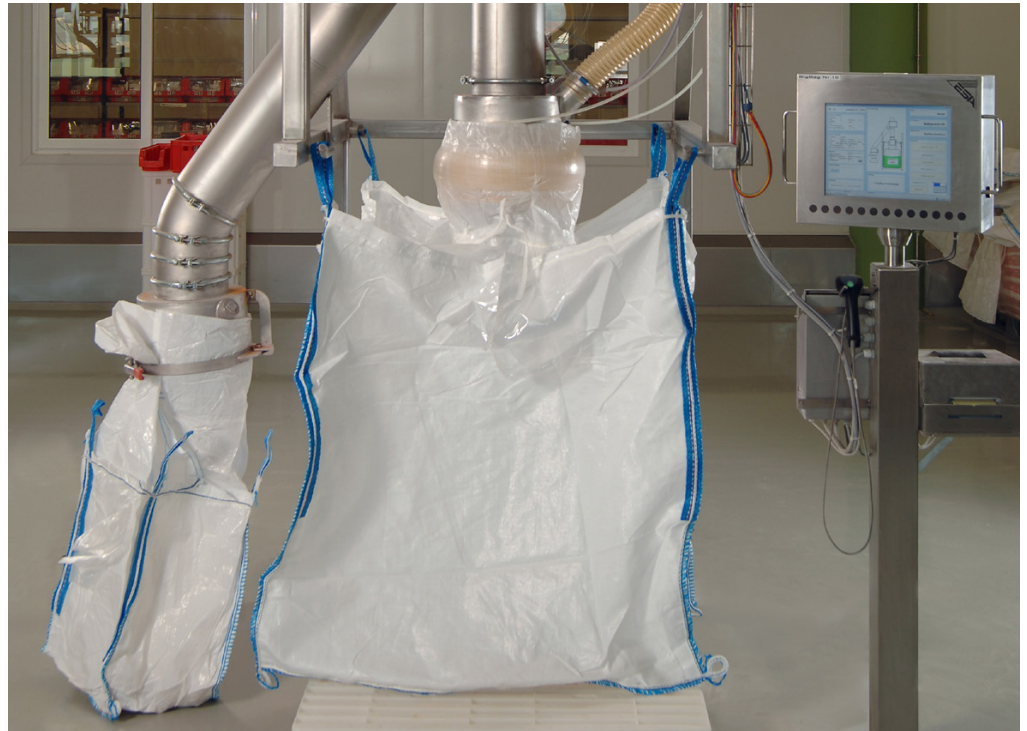
At „Almi“ IFS compliant metal detection is performed directly before filling of the spice products in bigbags.
