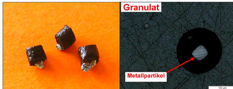
Regenerated plastic material (industry-grade material) containing metal contaminations. X-ray analysis (right picture) shows a metal particle that is completely embedded in the granulate.
