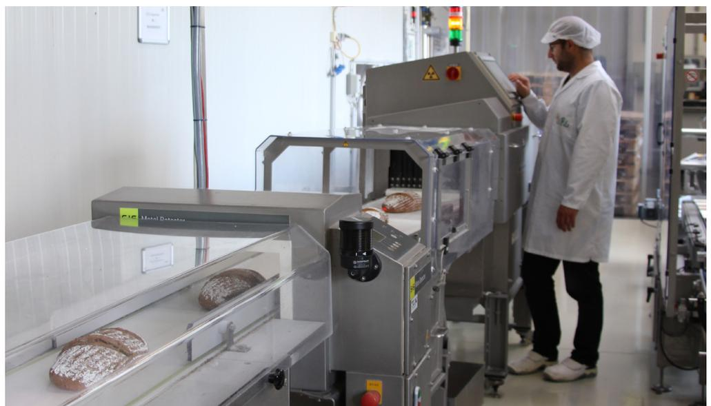
Sesotec combination solution with metal detector and X-ray system in the baking line of the company Backwelt Pilz.
