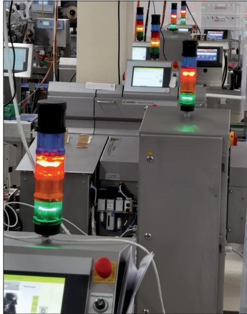
RAYCON EX1 x-ray inspection devices operating in nine lines: seven devices at FF Frischfleisch AG and two at Sempione AG
