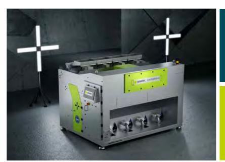
Application for sorting flakes and regrind materials in plastic recycling
